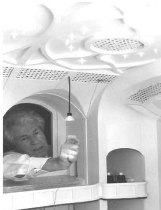
**Fig. 11: Measurements in the model of Landau Hall here with a little mirror reflector using laser as a point source**
