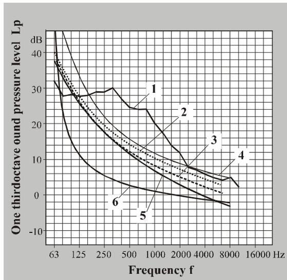
**Fig. 15 Air conditioning noise levels**
