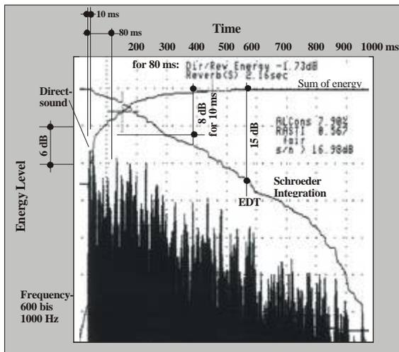
**Fig . 4 Impulse diagram of Landau Festival Hall with energy ratios and indexes, reverberation times and decay curve**
